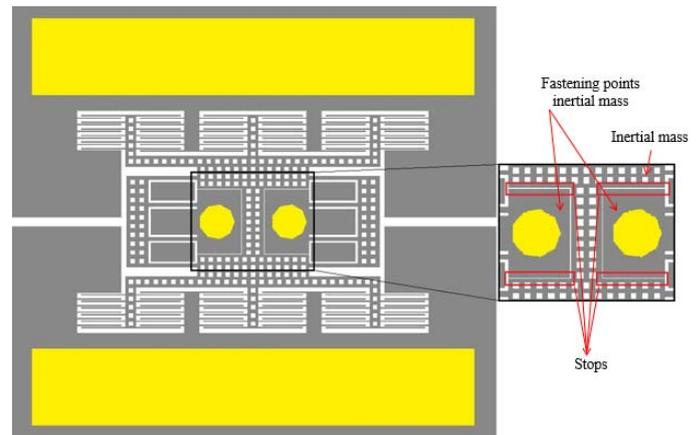
Fig. 5. The design of the MEMS-accelerometer “stoppers” elements.
