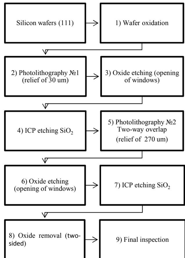
Fig. 1. Technological route of MEMS sensor element manufacturing.
