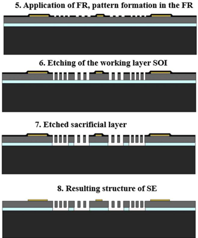
Fig. 2.2. Main technological operations of MEMS accelerometer sensor element manufacturing.
