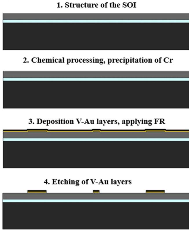
Fig. 2.1. Main technological operations of MEMS accelerometer sensor element manufacturing.
