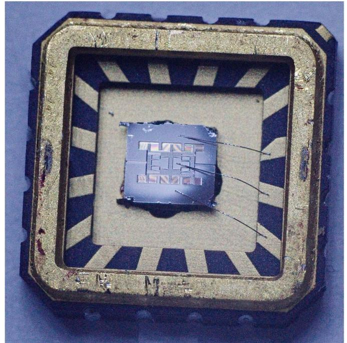
Fig. 4. MEMS sensor element in a package.
