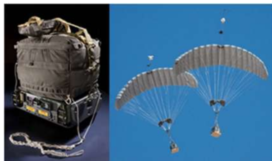
Fig. 2. Reusable JPADS-series system in stacked form [2] and in flight [4]
